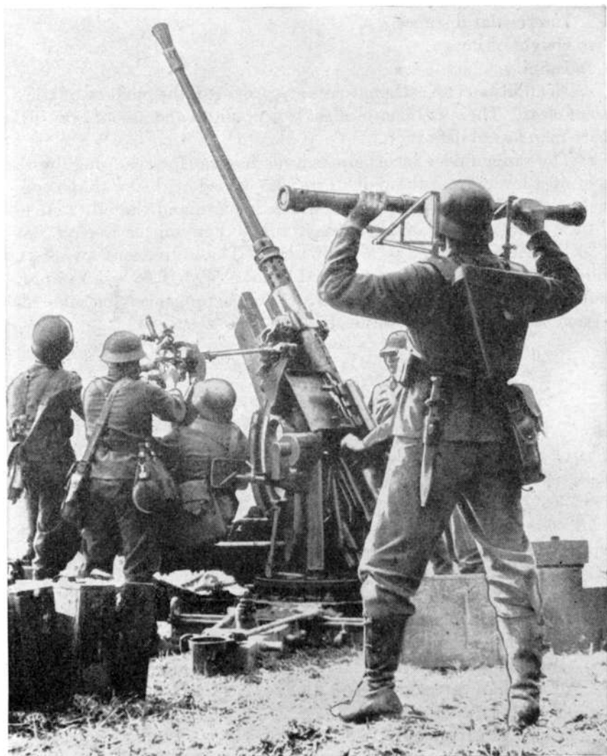
FIGURE 50.—1-meter-base range finder in use with 3.7-cm Flak 36 (37-mm anti-aircraft gun, single-barreled mount).
