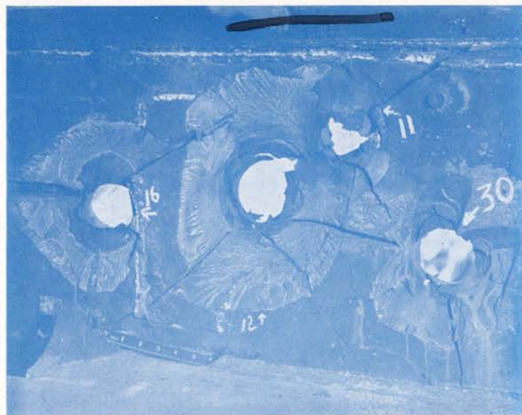
BACKSPALLS FROM 3" PROJECTILE, APC, M62, AT 0° OBLIQUITY, ON 4.05" UPPER HULL PLATE OF PzKw VI TANK. RANGES VARIED FROM 810 YARDS TO 1,640 YARDS.
