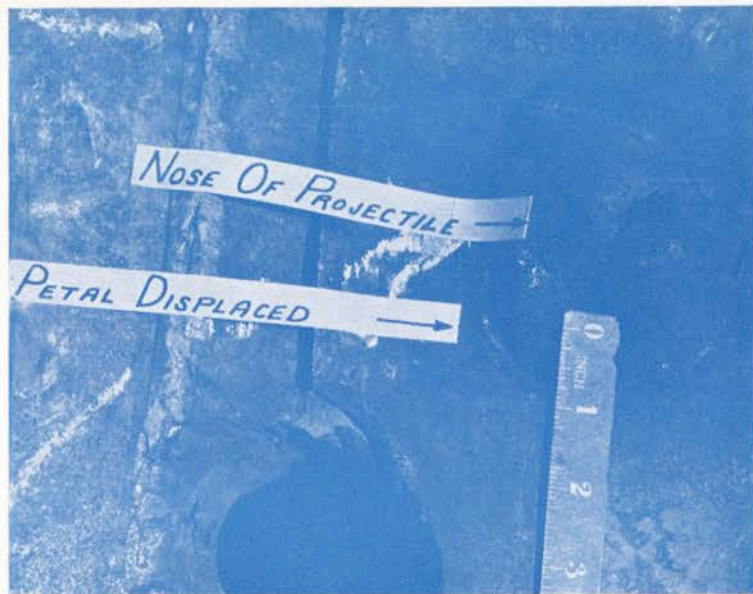
EFFECT OF 57MM PROJECTILE M86, ON 3.22" TURRET ARMOR OF PzKw VI TANK. OBLIQUITY WAS 0°. THE RANGE WAS 1,200 YARDS.
