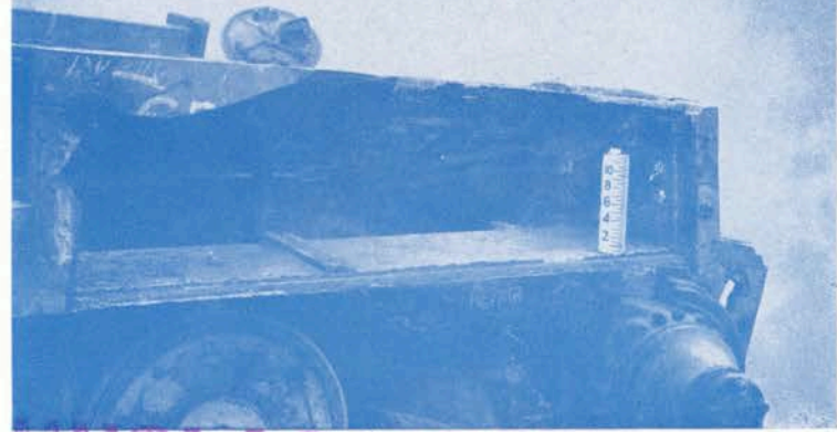
OPENING 62" x 27" CAUSED BY DISPLACEMENT OF SIDE ARMOR 3.22" THICK ON PzKw VI TANK CAUSED BY 3" PROJECTILE APC, M62. THE OBLIQUITY WAS 0°, AND THE RANGE WAS 2,530 YARDS.
