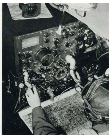
Shoran bombardier talks pilot onto drift arc of Shoran course and down bomb run. Pilot also gets PDI information on the run
